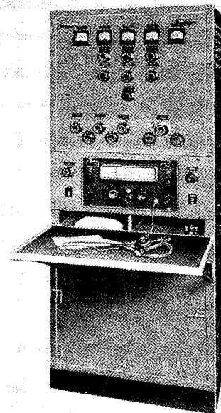
The complete ship's short-wave transmitter and receiver.
